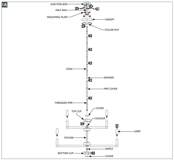
Screw the nipple to the bottom of the fixture, then place the bottom cup over the nipple and secure it in place by screwing the cover onto the nipple.
