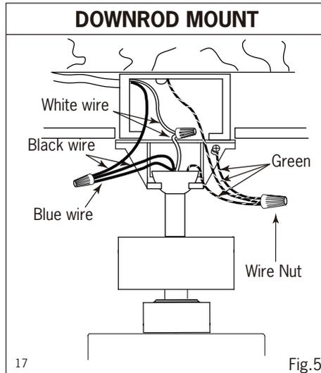
**NOTE:** Once ground wires are connected, carefully tuck all wires and wire nuts into the metal outlet box making sure that the wires are clear of the hemisphere and downrod when positioned in mounting bracket.
