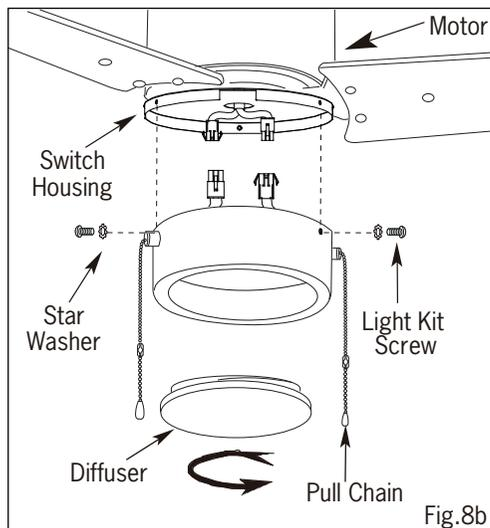
**WARNING: Ensure that all connections, set screws and screws are securely tightened before the next step.**
