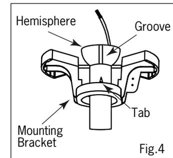
**NOTE: When installing fan on sloped ceiling, make sure tab on hanger bracket faces towards the top of the slope. Depending on the slope, a longer downrod may be required to prevent fan blades from hitting the ceiling.**
