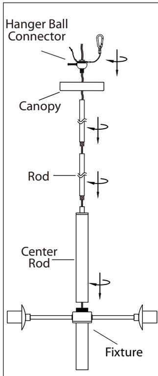
**1.** Screw the center rod to the fixture. Install the length of rod that is required by threading wire through the rod and screwing it to the fixture.
