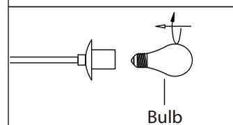
**8.** Install specified bulb type and wattage (not included).
