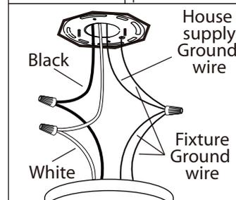
**5.** Connect the ground wires (bare copper or green) from your fixture to the ground wire (bare copper or green) or ground screw in the electrical box. Connect the black wire from the fixture to the black wire in the electrical box and connect the white wire from the fixture to the white wire in the electrical box.
