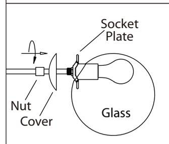
**9.** Insert the socket plate into the glass shade as shown.
