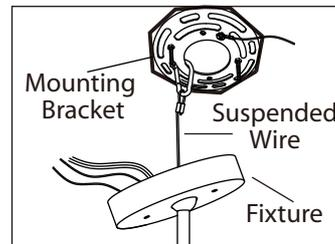
**4.** Use the suspended wire to hang the fixture as shown for wiring connection.
