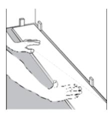
3. At the end of the first row, leave an expansion gap of 1/4" to the wall and measure.
