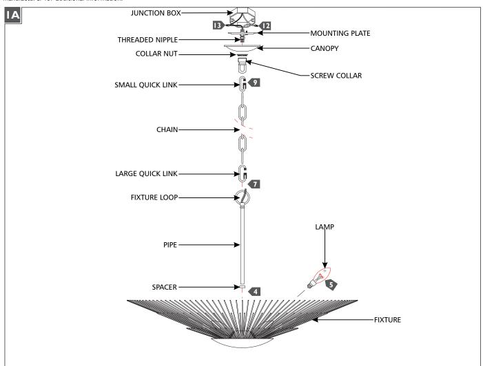
If necessary, screw the short end of the threaded nipple tightly onto the mounting plate.
