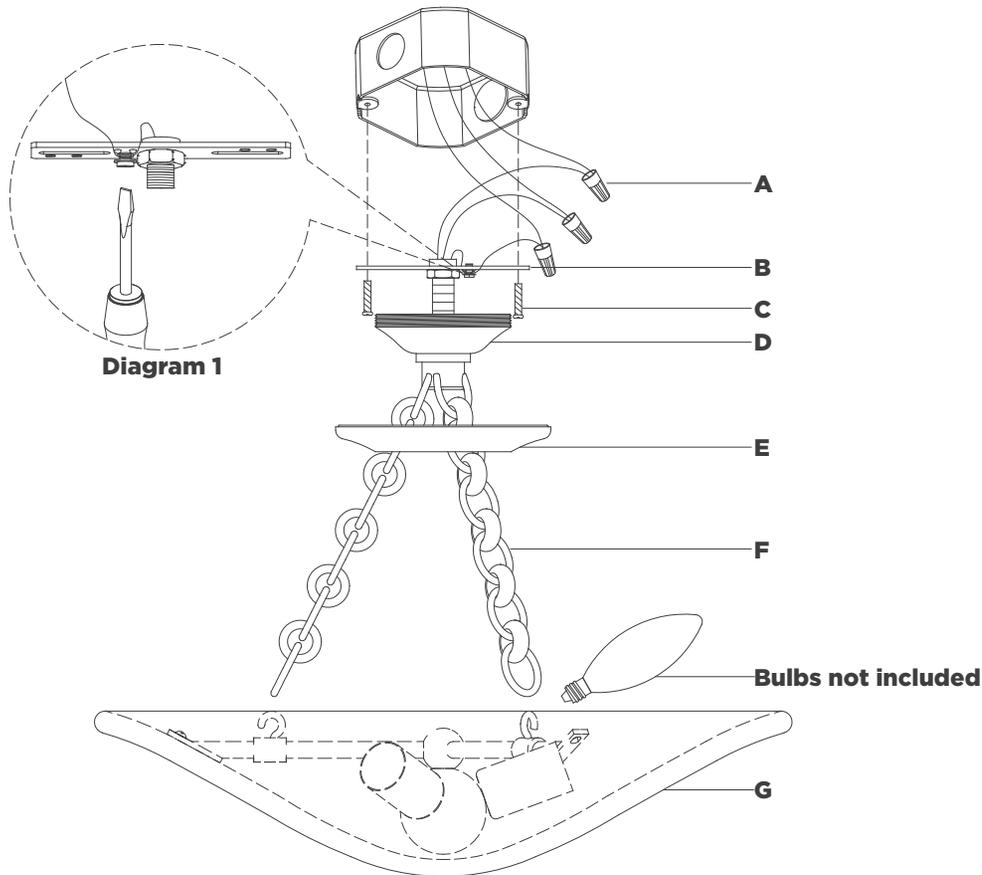
10. Wrap fixture ground wire (bare copper) around the green grounding screw (see diagram 1). Tighten. Continue fixture ground wire and connect to supply ground wire (usually green or bare copper) using wire nut **(A)**.
