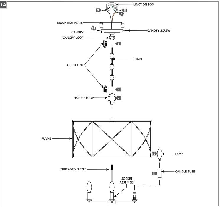
I Secure the mounting plate to the junction box.
