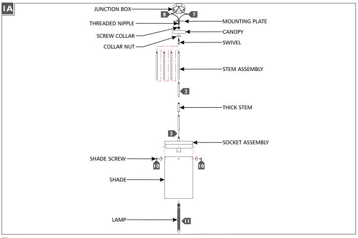
if necessary, screw the shorter end of the threaded nipple tightly onto the mounting plate, then screw the screw collar tightly onto the mounting plate.
