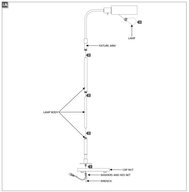
Install the base to the lower lamp body and secure them together using the washers and nuts with the wrench.
