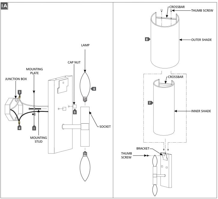
**1** Secure the mounting plate to the junction box.
