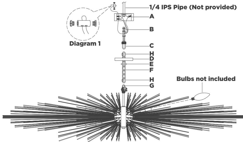
16. Install canopy **(D)** to collar loop **(C)** and secure with collar ring **(E)**.
